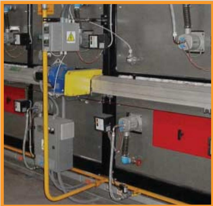
*The combustion system of Welko kilns is based on the already widely consolidated system of fixed air and modulated gas for temperature adjustment inside the kiln.*
